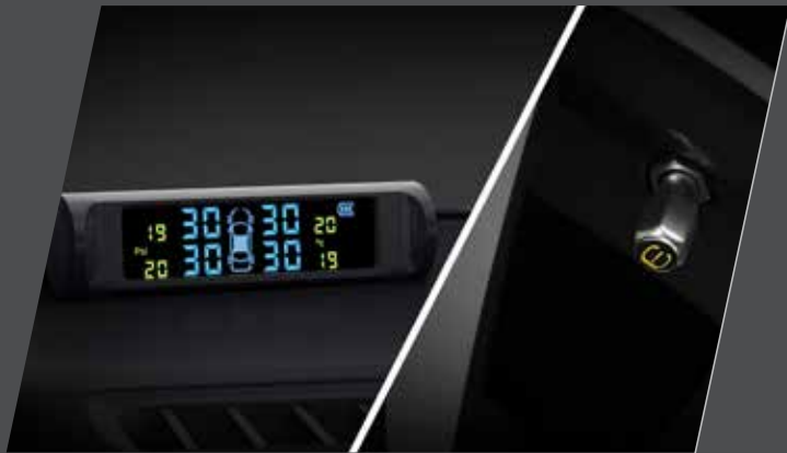
Tire-pressure monitoring system (TPMS) Keeps track of tire pressure wherever you go
