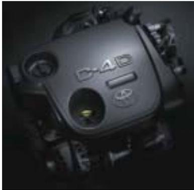
Newly Developed 1.5 L, 16 valve DOHC engine with a mileage of 17.6 Km / Lit [As per test agency under Rule 115 of CMVR, 1989]
