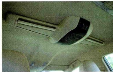
Roof blower is all about cabin air circulation
